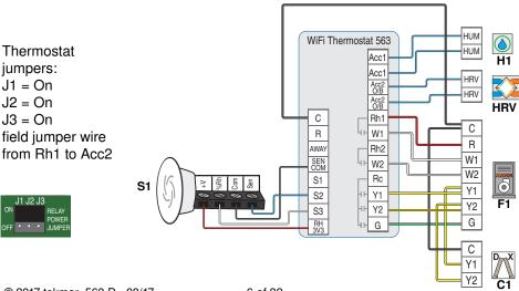
The WiFi Thermostat 563 operates a first stage radiant floor and a second stage fan coil for heating, and two-stage air conditioner for cooling and dehumidification, and a humidifier.
