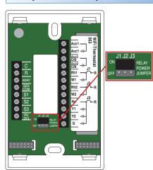
The thermostat includes three relay power jumper connectors located below the wiring hole.
