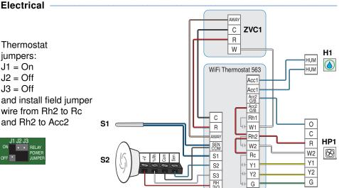
The WiFi Thermostat 563 operates a two-stage water-to-air heat pump for heating and cooling. The heat pump absorbs or rejects heat to a hydronic water loop that is heated by a boiler and cooled using a cooling tower to maintain a constant temperature of approximately 70°F (21°C).
