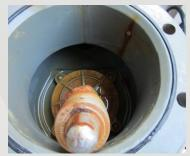
These images taken after 16 months in the same application as above shows little to no corrosion. Any corrosion resulting from a breach in coating has not spread.
