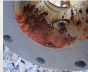
In these images taken 14 months after installation you can see many of the tubercles common to MIC and extensive corrosion.
