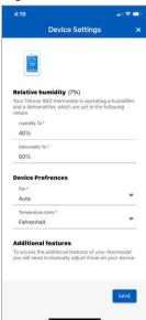
The Device Settings set the temperature units, fan, relative humidity and floor setpoints.
