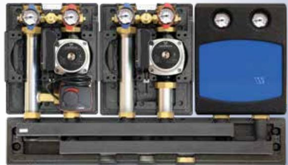
The ThermalPro™ boiler connection station is a modular, compact, pre-piped mechanical system complete with circulator, isolation ball valves, thermometers, pressure bypass valve and, on mixed stations, a 24 volt, 3-way mixing valve.
