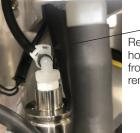
Remove plastic hose clamp from elbow, then remove tubing.
