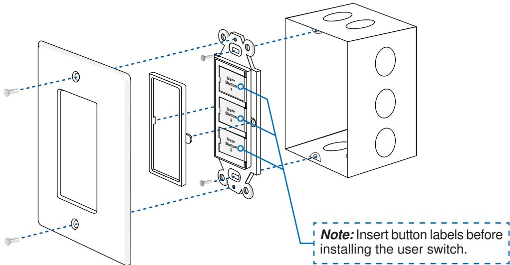
**Note:** Insert button labels before installing the user switch.
