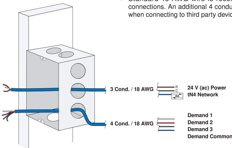
**Note:** When multiple wires run to the same equipment location, wiring conductors can share one wire jacket.
