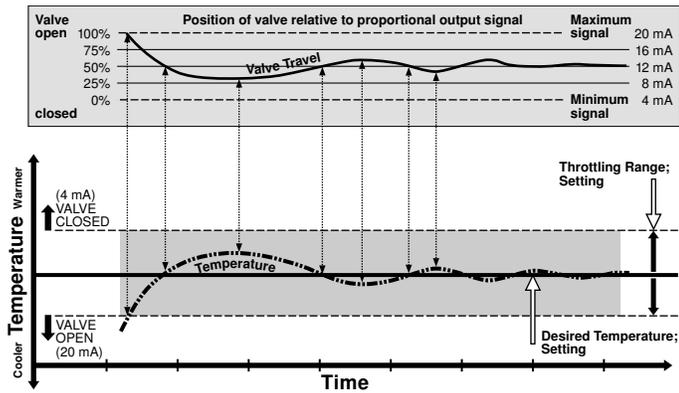
Fig. 9 Modulating, 4 to 20 mA function
