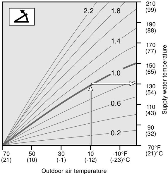
Fig. 2 Heating Curve
