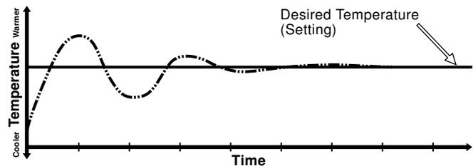
Fig. 5 Proportional + Integral + Derivative function
