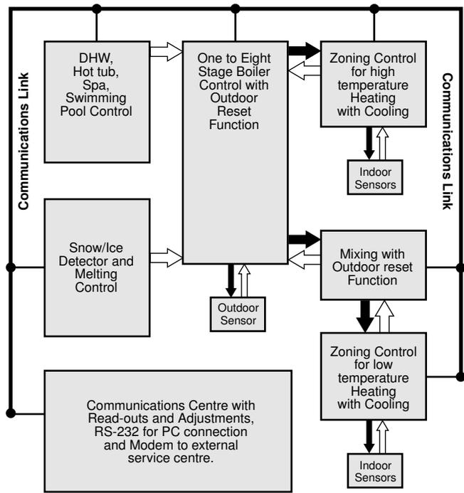
Fig. 10 Communications between Management Controls
