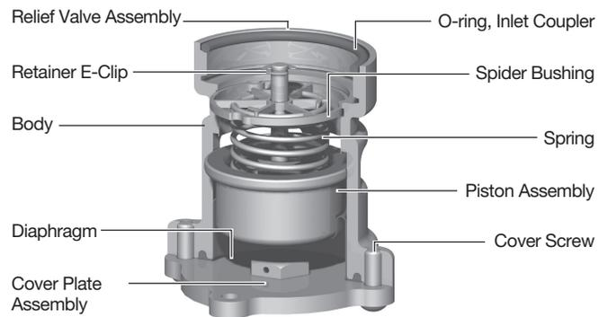
For repair kits and parts, refer to Backflow Prevention Products Repair Kits & Service Parts price list PL-A-RP-BPD found on [www.amesfirewater.com](http://www.amesfirewater.com).
