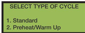
Use the **UP/DOWN buttons** to highlight the desired heat cycle. Press the **START button** to select the desired heat cycle.
