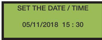
With the keypad (*see page 25*), enter the correct date using the MM/DD/YYYY format and the correct time using the 24 hour (military) format. Press **START button** to save the information entered and return to the Basic User Menu.
