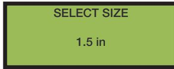
Use the **UP/DOWN buttons** to scroll through the list of available sizes. When you get to the size that you want, press the **START button** to confirm the selection.
