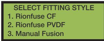
Use the UP/DOWN buttons to highlight the desired fitting style. Press the START button to select the desired fitting style:
