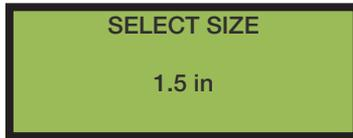
Use the **UP/DOWN buttons** to scroll through the list of available sizes. When you get to the size that you want, press the **START button** to confirm the selection.
