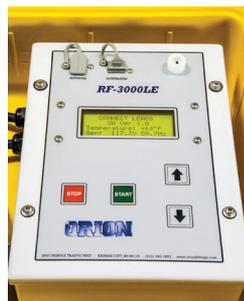
On the CONNECT LEADS screen, the second line indicates the major firmware version of the processor, in this case version 1.0.
